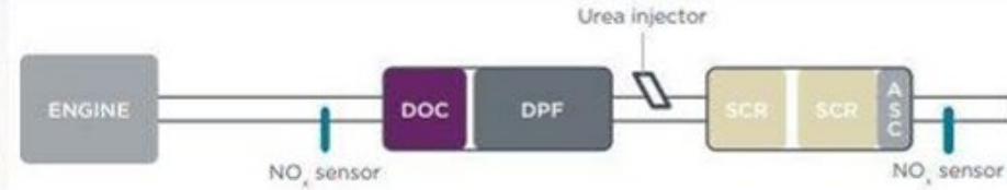
Figure 1. EPA 2010 aftertreatment system layout.
